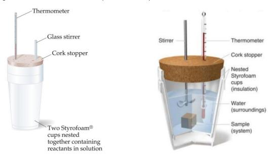
According to the Law of Conservation of Energy, energy is neither created nor destroyed. It can be assumed that no heat is lost to the calorimeter or the environment outside the calorimeter.
