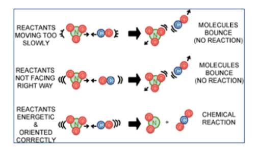
Sufficient Energy + Proper Orientation = Successful Collision
